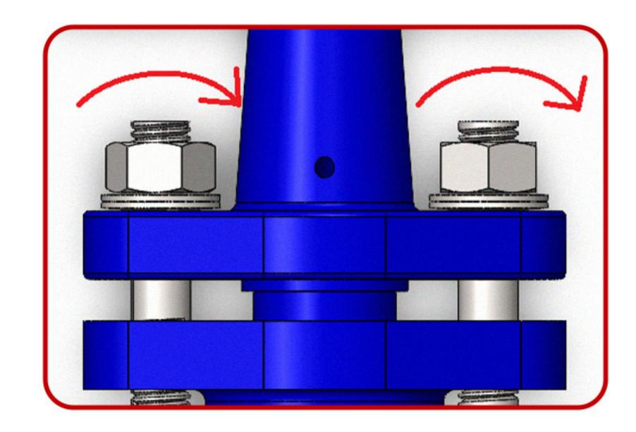
In case of any leakage observed on the piston valve we need to first close the piston valve and then tighten the bolts holding the body and bonnet. This will ensure further expansion of the sealing rings and will eliminate the leakage of the valve.
