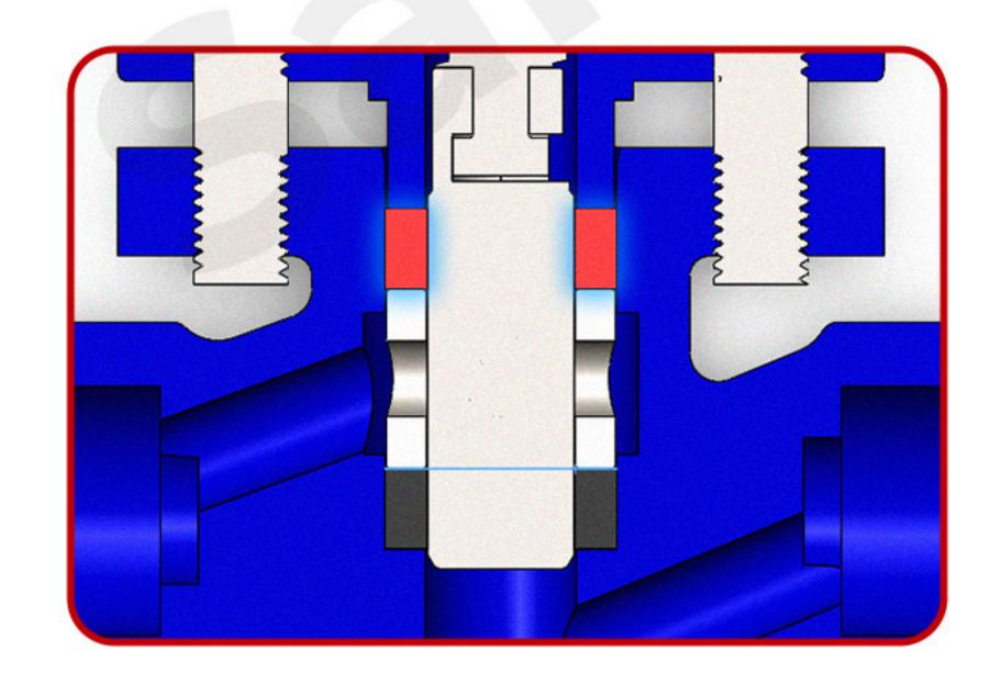
Replacement of the sealing rings should be done following proper replacement guidelines.
