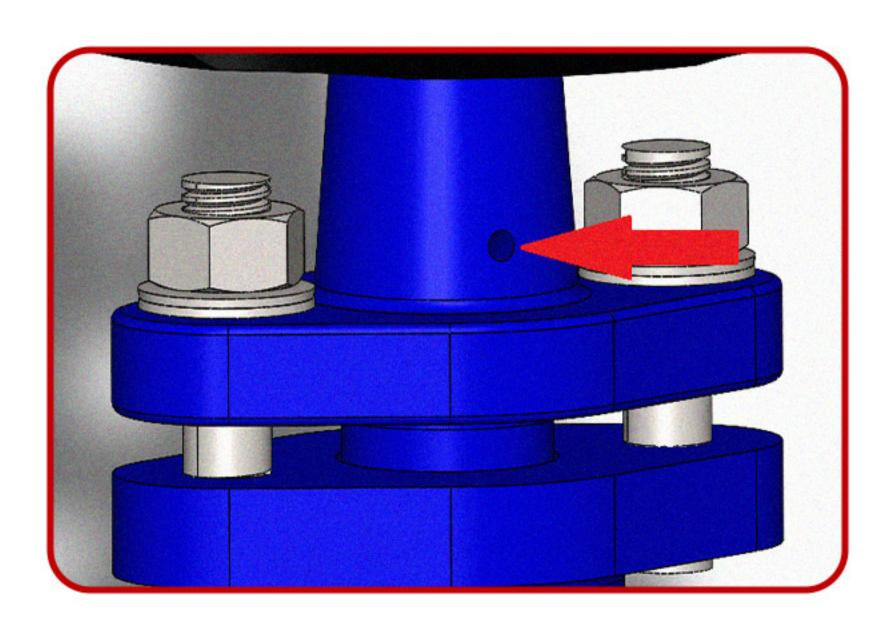
Piston valves have to be periodically lubricated with high temperature lubricant by applying the lubricant on the hole provided on the Bonnet of the Piston valve and also the spindle of the piston valve. After applying the lubricant we need to open and close the piston valves a couple of times to ensure proper spread of the lubricant.
