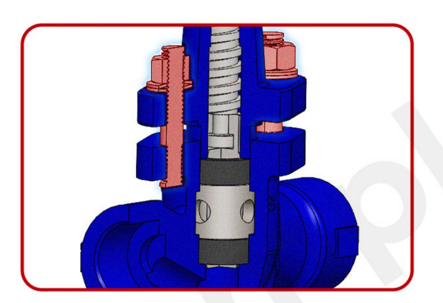
We should refrain from excessive tightening of the handwheel, as it can damage the sealing rings.
