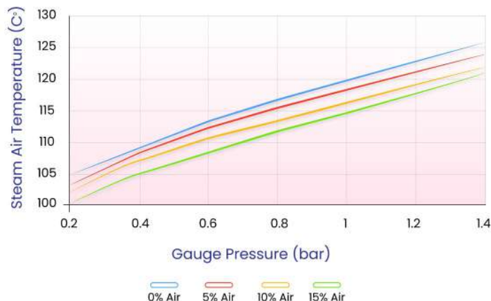
Mixture of Steam and Air Temperature vs. Pressure
